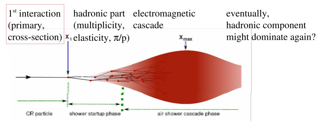
High numbers of low energy electrons excite  $N_2$  producing fluorescence light (detected isotropically) and charged particles emit Cherenkov (directionally)
