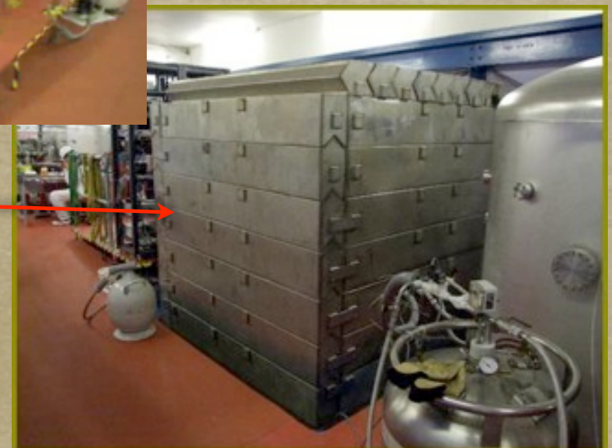
Steel encased 20 cm Pb gamma ray shielding
